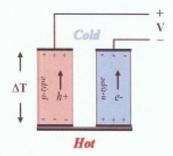
A complementary junction can be made of materials that use positive charge carriers, instead of electrons, to convey heat and charge away from the warm end. Connected beside a junction of the other type a complete circuit can be formed, or multiple pairs can be linked to increase the output voltage.
