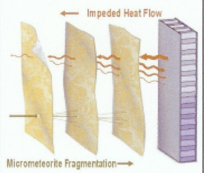
In addition to thermal control the MLI helps protect the spacecraft from micrometeorites. Incoming particles are shattered and lose energy as they penetrate MLI layers. The large spacing between New Horizons MLI layers serves to disperse the shower of penetrating debris over larger areas at the lower MLI layers, spreading out the impact energies.
